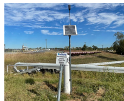
Installed tiltmeter station
