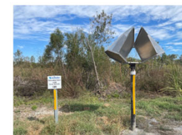
Installed InSAR corner reflector
