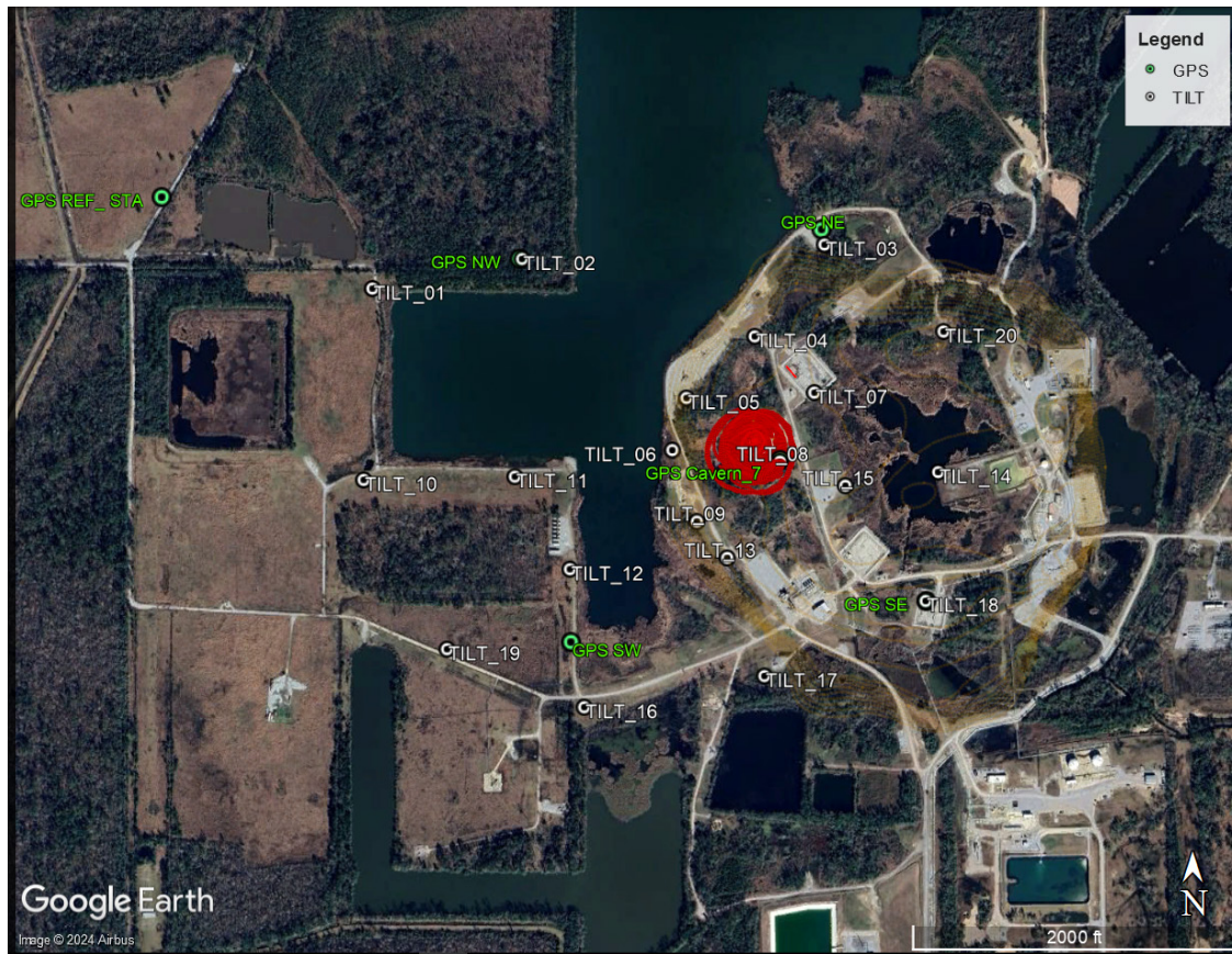
Figure 1. Google Earth image of Sulphur Mines salt dome with location of tiltmeters (white dots) and GNSS stations (green dots). Map includes the Cavern 7 sonar (red dots).
